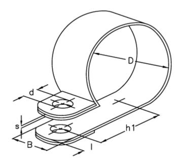
$\begin{array}{ll} d & = 10.5 \\ \text{Diameter D} = 44 \\ \text{h1} & = 36.5 \\ \text{I} & = 10.0 \\ \text{s} & = 1.0 \\ \text{Width B} & = 25 \\ \end{array}$
